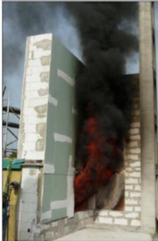
14th minute calibration test and test of ETICS with EPS
