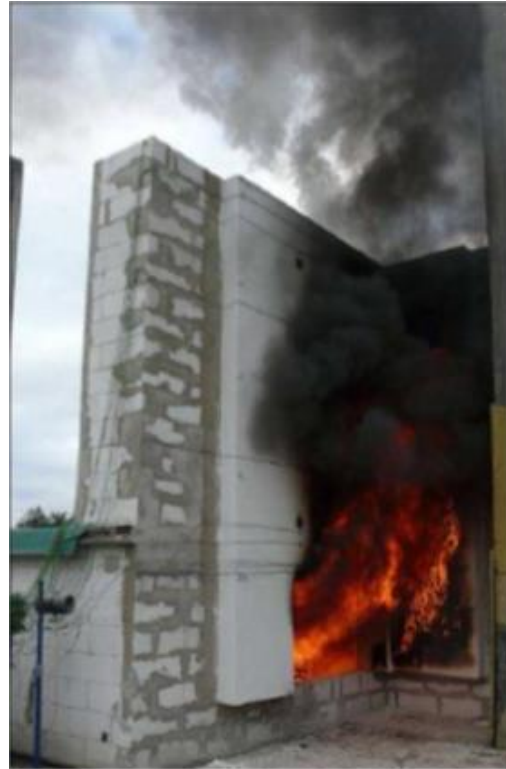
14th minute calibration test and test of ETICS with EPS
