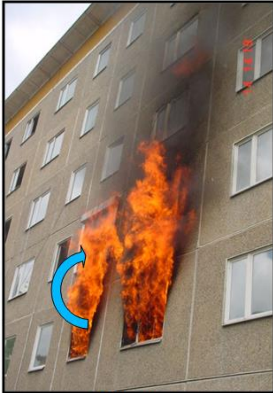
12th minute „flash-over“ 1st floor
