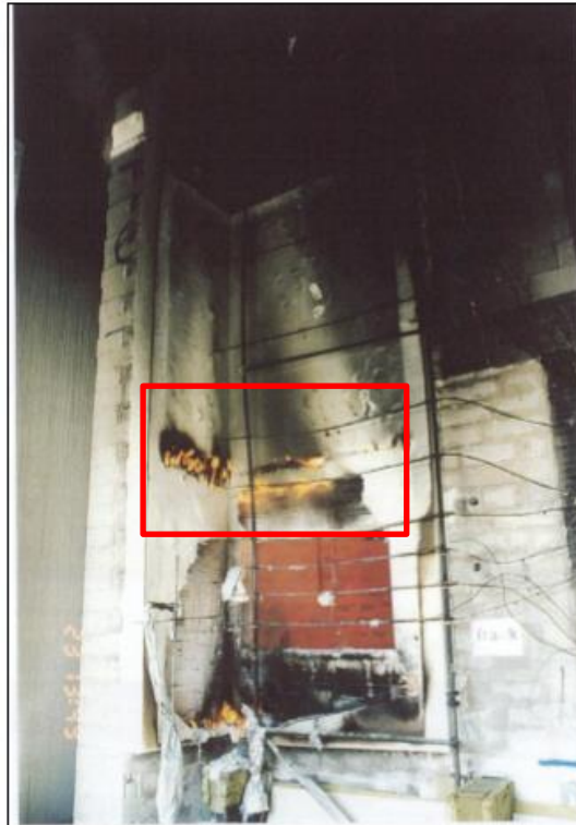
after 30 minutes - the flame did not spread the sample
